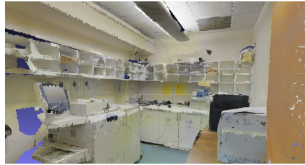
Figure 1. Visualization of raw point cloud of one of the copy rooms of area 5
